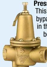
**Pressure Reducing Valve –** This valve, with built-in bypass, should be installed in the supply line to the booster to regulate and stabilize flow pressure to 20 psi.
