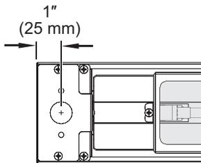
Distance from end of unit to center of conduit hole.
