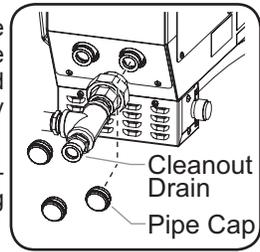
**NOTE:** Perform the entire "Daily Cleaning" procedure in the MAINTENANCE section of this manual if buildup is significant.
