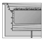
The unique angled inside wall design provides easy access and clear views. The greater surface area of the angled wall and the placement of the coils allow cold air to more effectively blanket your food product.
