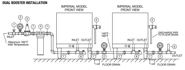
(1) ¾" Gate or Ball Valve\* (2) Temperature/Pressure Gauge (3) Pressure Reducing Valve with By-Pass (4) Blended Phosphate Water Treatment System (5) Relief Valve (must have discharge pipe to floor drain) (6) Shock Absorber (7) Union\* (8) Drain Pipe Valve\* \*Supplied by installer CONSULT LOCAL CODES
