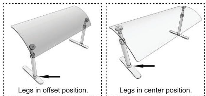
3. Install the vertical posts to the acrylic shield.
