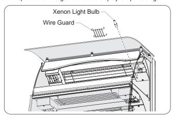
Replacing the Display Light Bulbs
