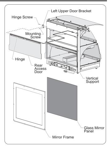
Installing the Rear Access Doors
