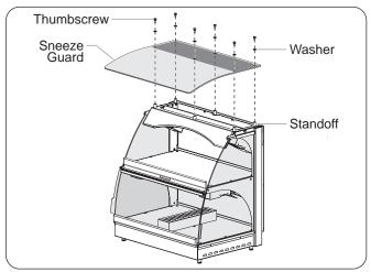
Installing the Sneeze Guard
