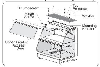
Installing the Upper Front Access Door
