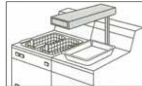
GRFS, GRFSL, GRFSC, GRFSL with swing-away post mount and cord with plug
