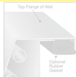
BEZELGASKET-2, -3, -4, -5, -6 Factory installed option (eliminates the need for silicone or other sealants)
